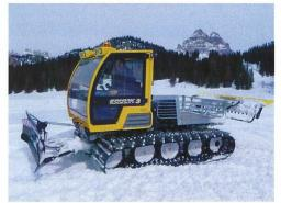
THE DRIVER'S CABIN, THANKS TO ITS LARGE WINDSCREEN, SLIDING SIDE AND REAR WINDOWS, PROVIDES OPTIMAL ALL-ROUND VISIBILITY, WHILE A PLEASANT LOW-NOISE ENVIRONMENT IS GRANTED BY MEANS OF VARIOUS INSULATING PANES.
